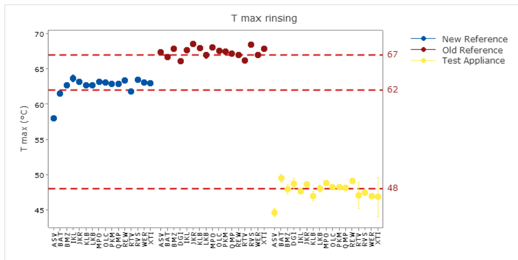
Figure 35: Mean values and SD of maximum temperature rinsing by lab and machine (detergent D+E)
